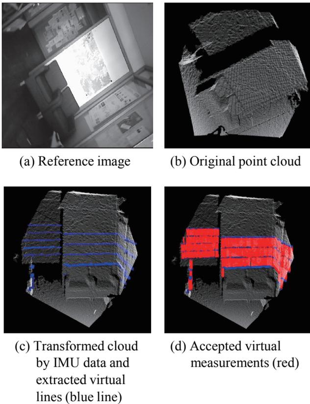
**Fig. 1** Extraction procedure of wall-like features.
