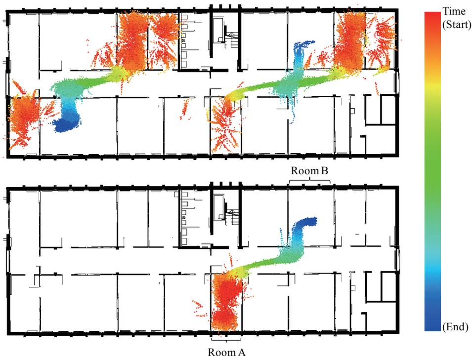
**Fig. 2** Trajectories of particles in the ambiguous environment. Localization result with uniform initialization (top). Localization result with WiFi based initialization (bottom). The color of the particles depicts the time transition. Our method uniquely localizes the target. The target moved from room A to room B.
