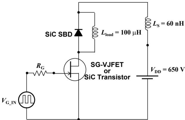
**Fig. 3** Diagram of a standard inductive load test circuit to evaluate the dynamic characteristics of the three transistors.
