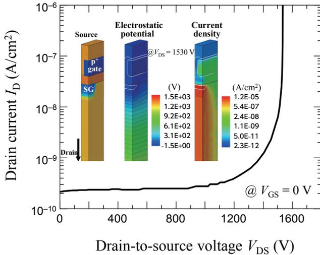
Fig. 6 Simulated forward blocking characteristic of SG-VJFET at  $V_{GS} = 0$  V.
