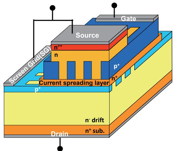
**Fig. 2** A schematic diagram of the proposed SiC VJFET structure (Screen Grid vertical JFET: SG-VJFET).
