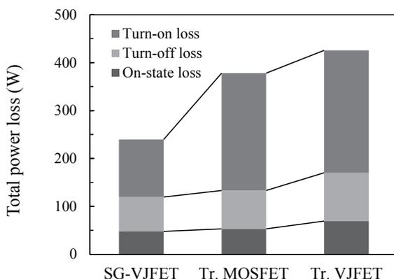
**Fig. 10** Comparison of FET total power loss among three different transistors. (Switching current: 400 A/cm<sup>2</sup>)
