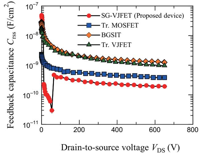
Fig. 7 Comparison of simulated feedback capacitance  $C_{iss}$  among three different types of SiC transistors.
