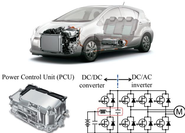
**Fig. 1** Power conversion system for hybrid electric vehicles (HVs). Power control unit consists of DC/DC converters, DC/AC inverters, passive components and liquid cooling system.
