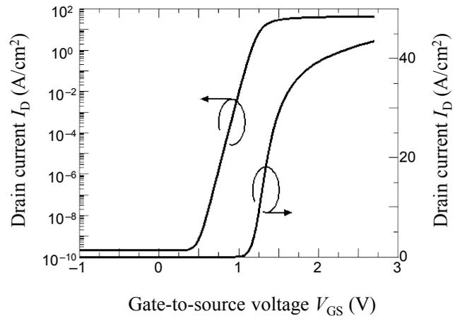
**Fig. 4** Simulated transfer characteristic ( $I_D$  vs.  $V_{GS}$ ) of SG-VJFET.
