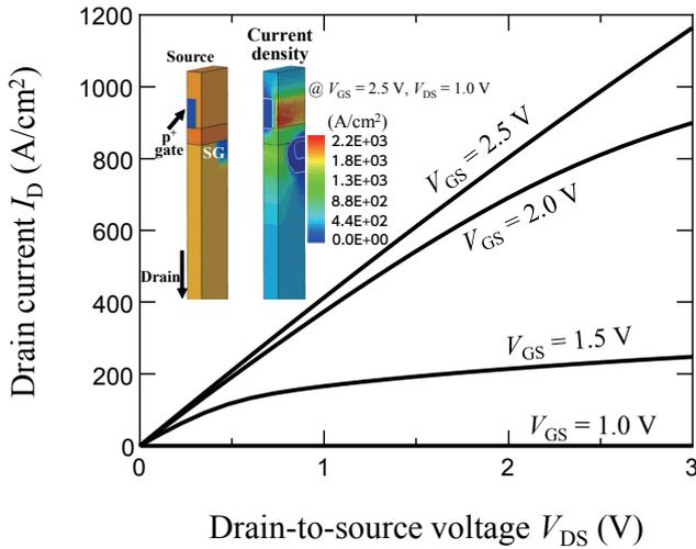
Fig. 5 Simulated output characteristic ( $I_D$  vs.  $V_{GS}$ ) of SG-VJFET at  $V_{GS} = 1.0$ - $2.5$  V.
