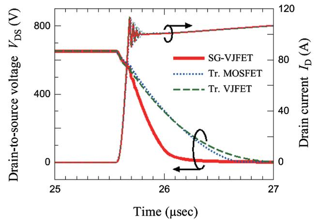
Fig. 8 Simulated turn-on switching waveforms of three different transistors. ( $V_{DD} = 650$  V,  $I_D = 100$  A)
