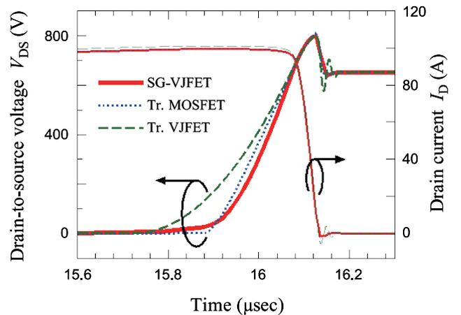
Fig. 9 Simulated turn-off switching waveforms of three different transistors. ( $V_{DD} = 650$  V,  $I_D = 100$  A)
