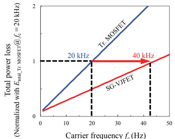
**Fig. 11** Dependence of total power loss on carrier frequency  $f_c$ . Each data is normalized with total loss of trench-gate MOSFET at  $f_c = 20$  kHz.
