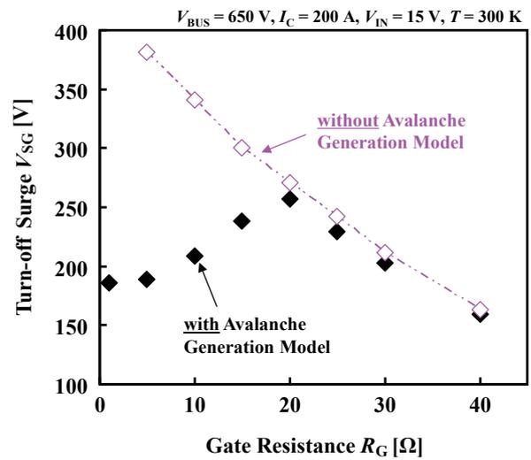
**Fig. 6** Simulated gate resistance dependence of turn-off surge with and without avalanche generation model.
