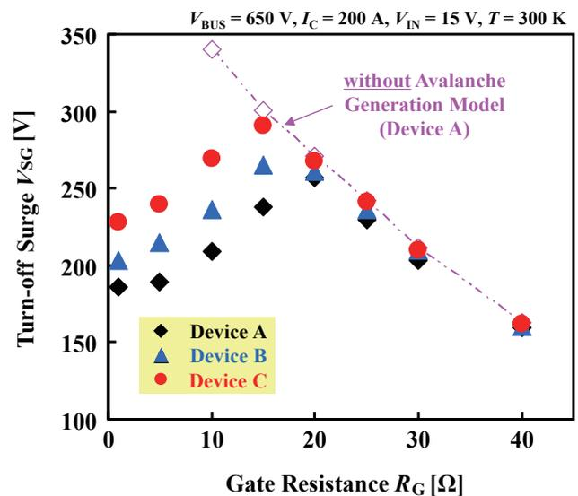
Fig. 9 Simulated gate resistance dependence of turn-off surge with each device.
