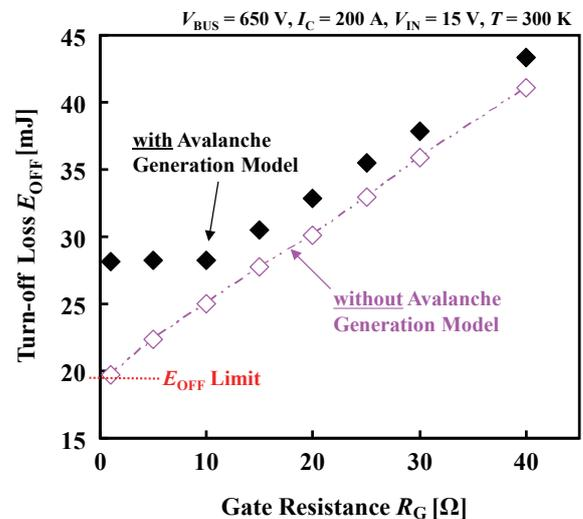
**Fig. 7** Simulated gate resistance dependence of turn-off loss with and without avalanche generation model.
