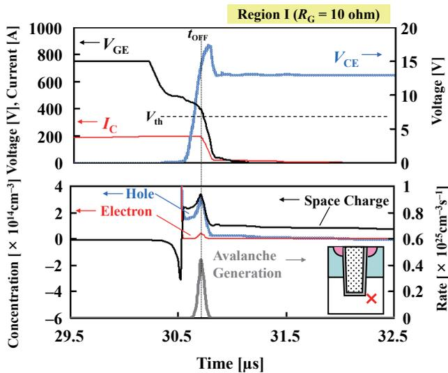
Fig. 3 Simulated switching waveforms and internal dynamics adjacent to bottom of trench for Region I.
