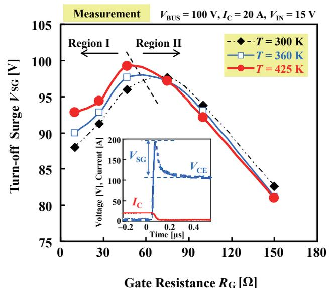
**Fig. 1** Measured dependence of turn-off surge on gate resistance and temperature. Inset: measured switching waveforms.
