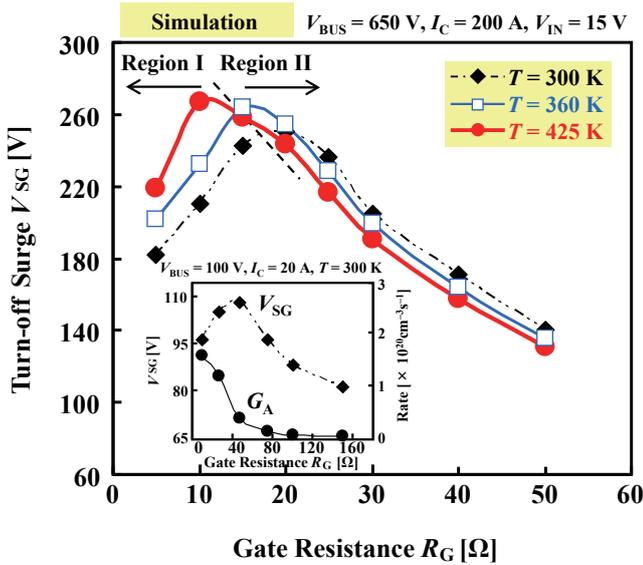
Fig. 2 Simulated dependence of turn-off surge on gate resistance and temperature. Inset: simulated dependence of avalanche generation rate and turn-off surge on gate resistance under the same circuit parameters in the measurements.
