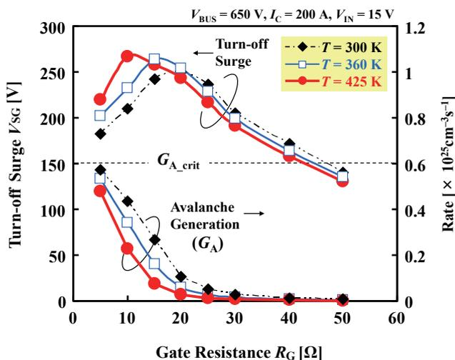
**Fig. 5** Simulated dependence of turn-off surge and avalanche generation rate on gate resistance and temperature.
