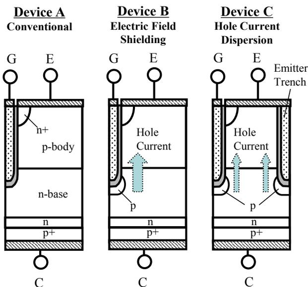
Fig. 8 Simulated device structures for suppression of dynamic avalanche near gate trench bottom.
