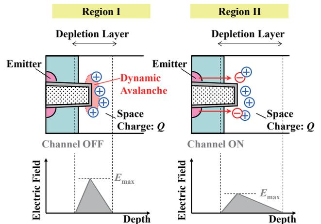
Fig. 4 Schematic diagram of internal space charges at each region just before collector current turn-off.
