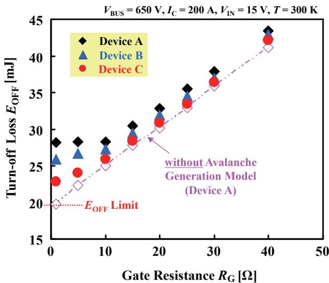
Fig. 10 Simulated gate resistance dependence of turn-off loss with each device.
