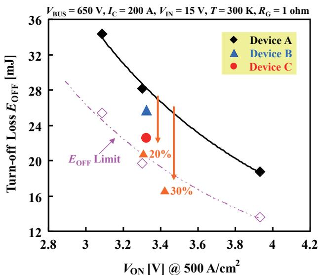
Fig. 11 Simulated trade-off relation between on-state voltage and turn-off loss with each device.
