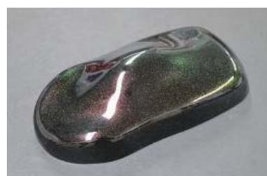
**Fig. 7** Photograph of a car-shaped model coated with clear paint that included the colloidal crystal flakes.
