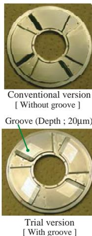
Fig. 4 Test pieces of compliant foil thrust bearing.
