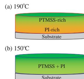
**Fig. 3** Structures of PTMSS/PI bilayer thin films. (a) Annealed at 190°C. An interface is left between the PTMSS-rich layer and the PI-rich layer. (b) Annealed at 150°C. PTMSS and PI interdiffuses into a mixed layer.
