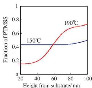
**Fig. 2** Cross-section profiles of the fraction of the component polymer. The change in the 190°C plot indicates the existence of an interface of about 30 nm in thickness. The constant fraction of 150°C represents the mixing of the polymers.
