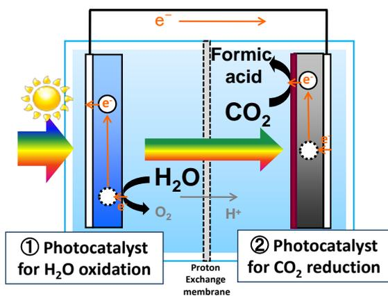
Figure 1. Schematic illustration of the artificial photosynthesis.
